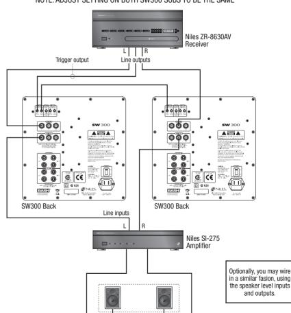
Figure 4. Stereo/dual subwoofer application
